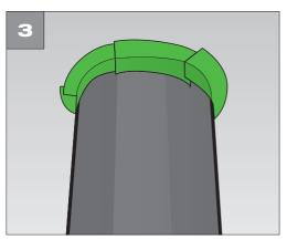
Apply Rissan around circular parts in layers
