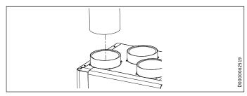
▶ Push the air duct over the air connector.
