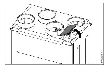
► Carefully lift up the control panel cover. The terminal block, from which cables lead into the appliance, is suspended from the underside of the cover.
