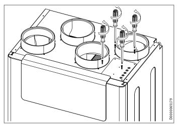
▶ Undo the four screws from the control panel cover.
